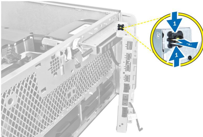
6. Remove the power switch from the computer.
