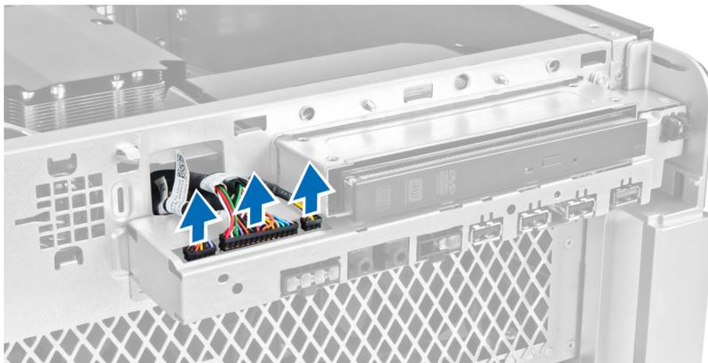
4. Remove the screws that secure the front I/O panel to the computer chassis.
