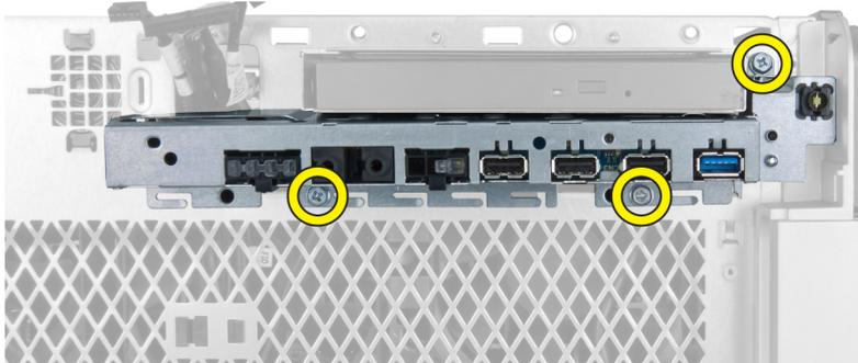
5. Pull the front I/O panel in a direction opposite to the computer to release its edge from the chassis clip.
