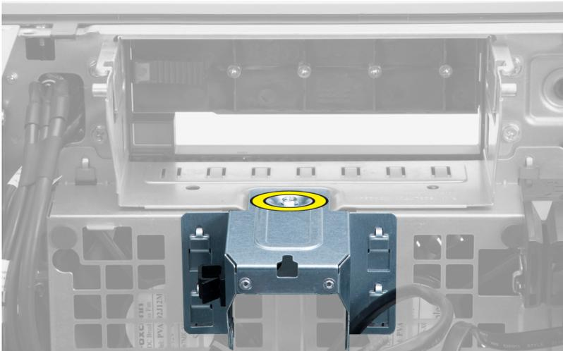
5. Press the latches on either side of the metal plate to release it.
