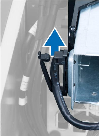
7. Lift up the release latch on top of the optical-drive cage.
