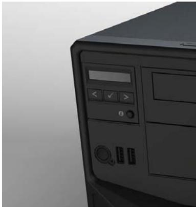
**Figure 10. LCD-Front Panel (Hot-Swap HDD Configuration)**
