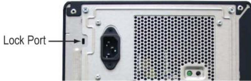
**Figure 14. Lock Port on Back of Chassis**
