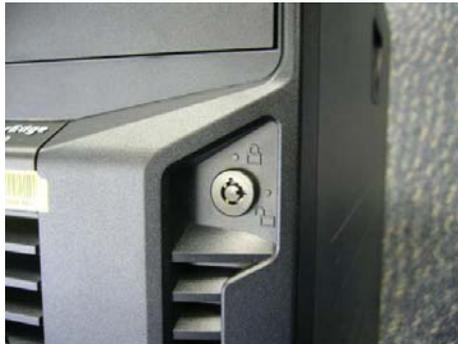
**Figure 13. Bezel Lock in Front Bezel**
