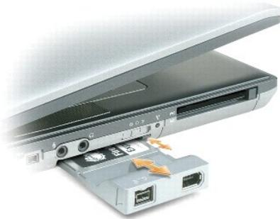
The computer recognizes most cards and automatically loads the appropriate device driver. If the configuration program tells you to load the manufacturer's drivers, use the floppy disk or CD that came with the card.
