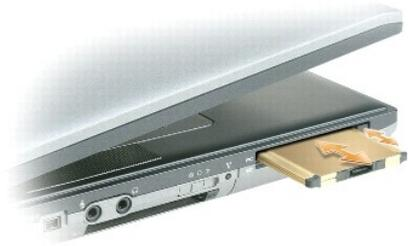
The computer recognizes most cards and automatically loads the appropriate device driver. If the configuration program tells you to load the manufacturer's drivers, use the floppy disk or CD that came with the PC Card.
