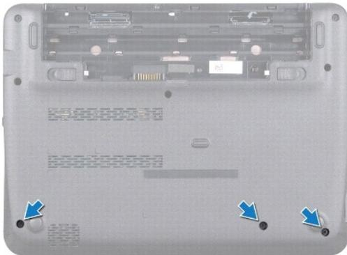
4. Remove the keyboard (see [Removing the Keyboard](#)).
