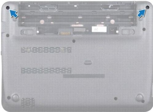
4. Using a plastic scribe, gently pry out the middle cover and remove it from the computer base.
