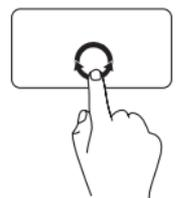
Move a finger in the horizontal scroll zone (extreme bottom of the touch pad), in a clockwise circular motion to scroll right or counterclockwise circular motion to scroll left.
