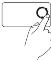
Move a finger in the vertical scroll zone (extreme right of the touch pad), in a counter clockwise circular motion to scroll up or clockwise circular motion to scroll down.
