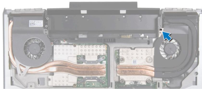
9. Disconnect the processor fan and heat sink assembly cable from the system board connector.
